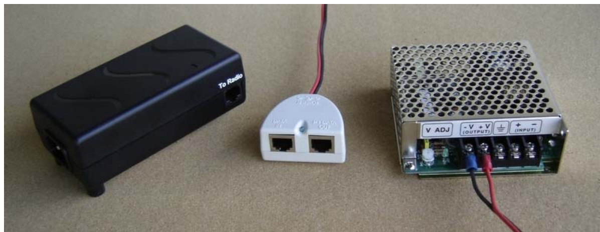
Figure 1.2 – Power Inserter Units and DC/DC Converter
